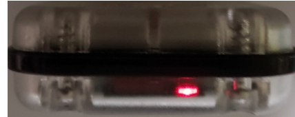
End view of tag showing magnetic reed switch and LED
