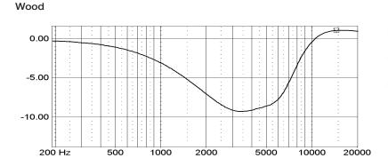
F1=3.43khz, -9.1dB, Q=0.79, BW=1.27 Oct F2=5.76khz, -6.1dB, Q=1.49, BW=0.67 Oct F3=11.3khz, +5.55dB, Q=1.24, BW=0.8 Oct
