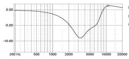
F1=3.4khz, -9.3dB, Q=1.4, BW=0.71 Oct F2=6.42khz, -7.6dB, Q=1.47, BW=0.68 Oct F3=9.48khz, +6.4dB, Q=1.19, BW=0.84 Oct
