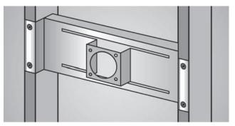
Figure 2 SolidDrive MSK-1-T mounting bracket attached to the wall studs
