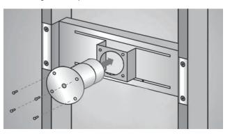
Figure 3 SolidDrive MSK-1-T being installed into the mounting bracket
