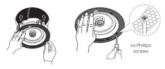
**6** Reposition the grill on the loudspeaker.
