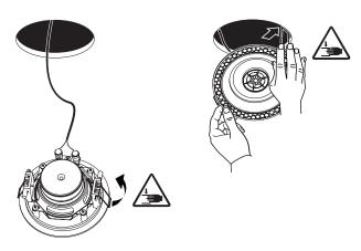
6 Lift the other clamp and insert in into the hole in order to set the loudspeaker in its final position.
