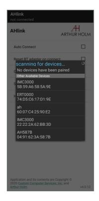
Selecting the device, the first page will load on the mobile phone. This page is used to check the device. When the mobile APP is connected to the unit, the RF LED will be on. The name always begins by "ERT" characters followed by the fourth last digits of the serial number. Select the device to control and configure the unit.
