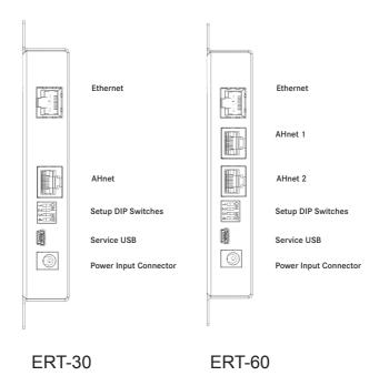
**ETHERNET:** RJ45 network connector. Connect the ERT to your local network, to open the 2002 port and send AHnet commands to the units connected to the RS422/RS485 Full Duplex ports (AHnet1 and AHnet2).
