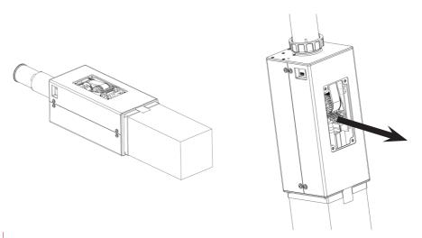
Remove the cable bag from the unit by pressing the 2 tabs. Then pull the cable and remove it.
