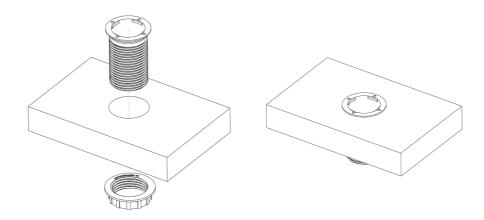
Tighten the nut until the upper ring of the support is completely flush with the surface of the table.
