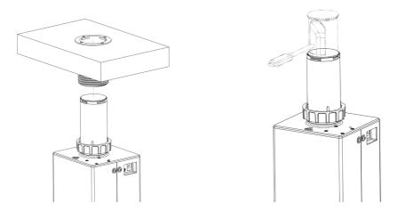
Tighten it by hand, by holding the unit on the position, with one hand, while screwing the unit nut with the other one.
