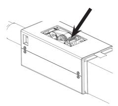
To ensure the cable is not blocked, pull slightly the cable through the output head and check that the drive belts rotate correctly.
