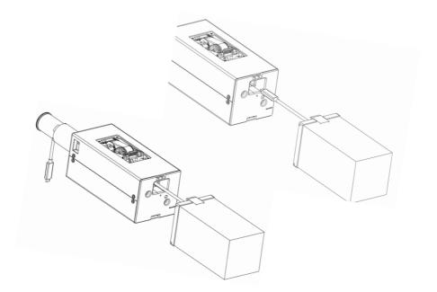
Close the cable traction system by pushing from the tab.
